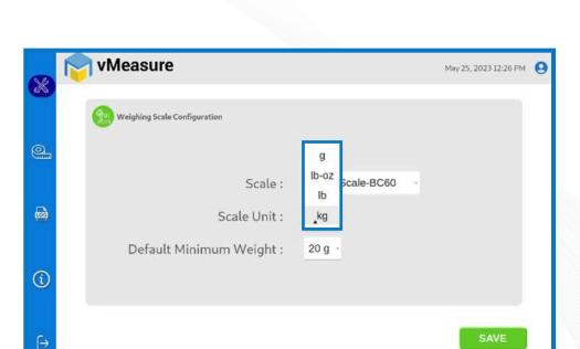
Step 3.2: Scale Unit: Choose the unit that is displayed on the weighing scale.
