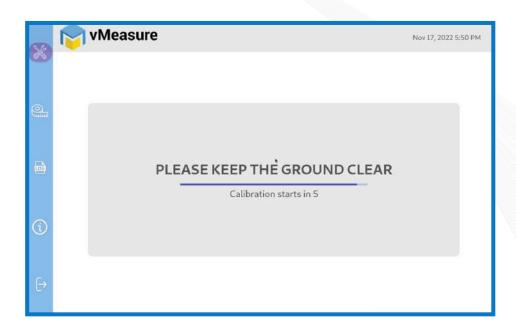
**Step 6:** Wait for 5 seconds for the system to calibrate.
