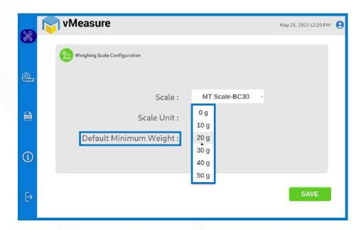
Step 3.3: **Default Minimum Weight:** Select the minimum weight that needs to be displayed by default when the actual weight of the product is very light.
