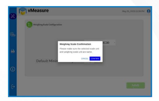
(i) The unit selected should match with the unit configured on the weighing scale.
