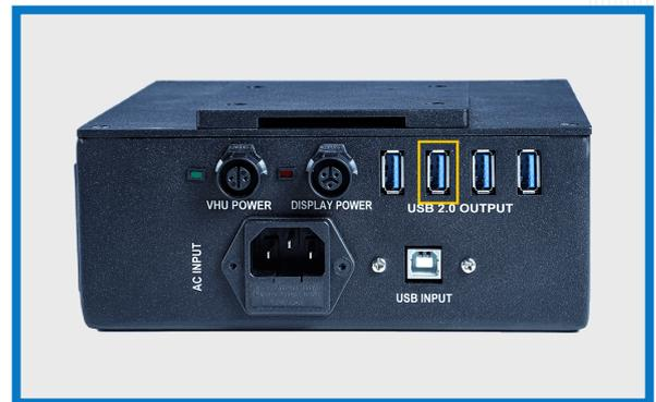
Step 1: Connect the weighing scale to vMeasure Parcel Ultima.
