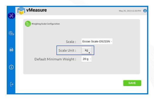
Step 3.2: Scale Unit: Choose the unit that is displayed on the weighing scale.
