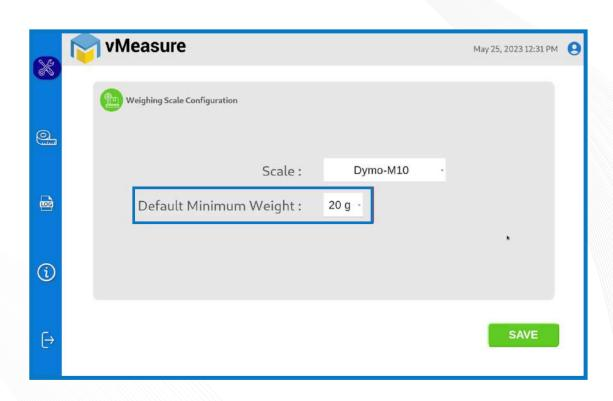
Step 3.2: **Default Minimum Weight**: Select the minimum weight that needs to be displayed by default when the actual weight of the product is very light.
