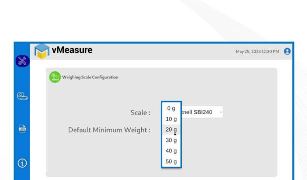
Step 3.2: **Default Minimum Weight**: Select the minimum weight that needs to be displayed by default when the actual weight of the product is very light.
