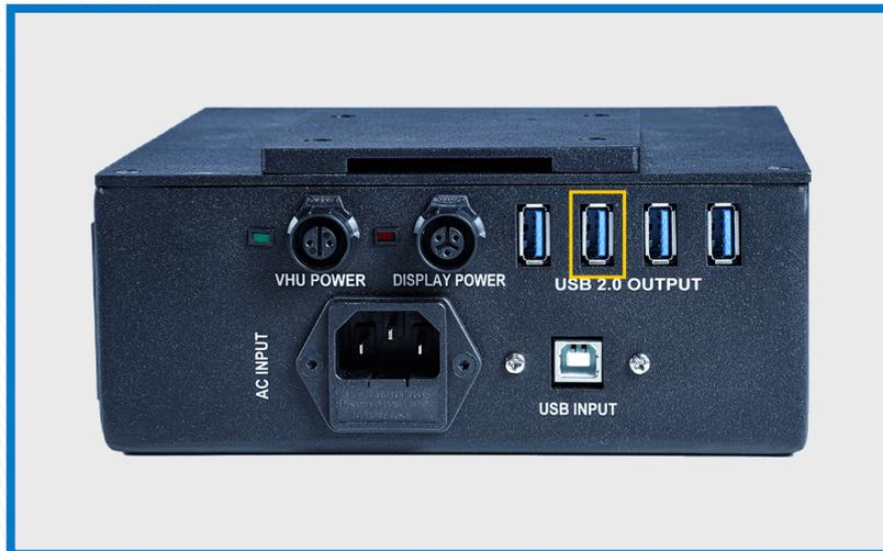
**Step 1: Connect the USB from the weighing scale to one of the USB ports of the Power Box and plug the power cable to a main power source**
